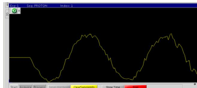
**Figure 2** Low frequency sine wave: Z0 close to correct setting. Minimize frequency by clicking the Z0 button in +/- 100 mode or clicking and holding button in +/- 10 mode.
